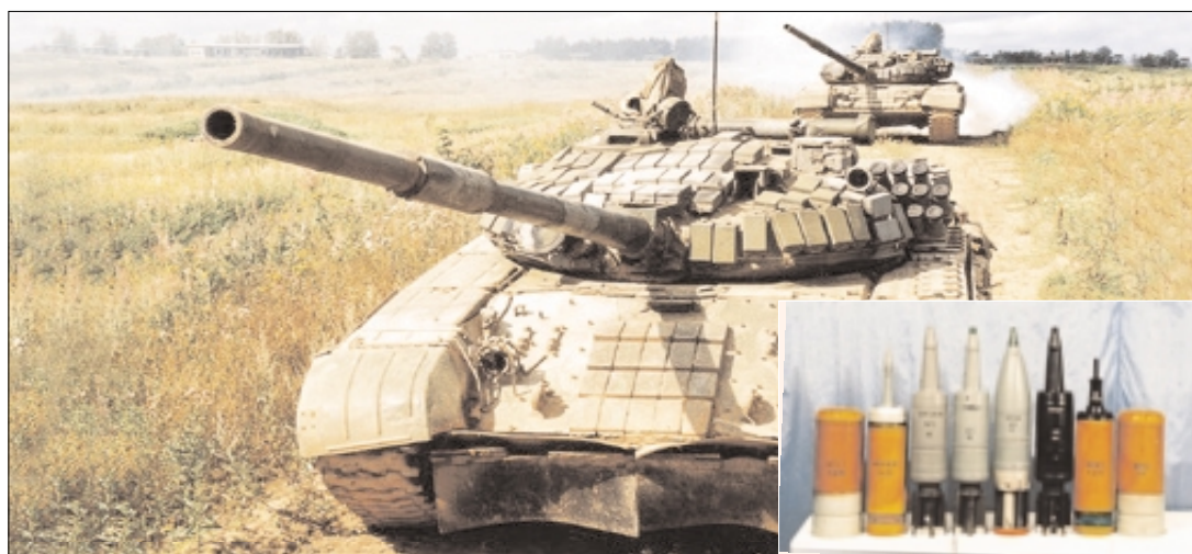
125mm 3VBM17 ROUND WITH 3BM42 APFSDS PROJECTILE FOR D-81 GUN
