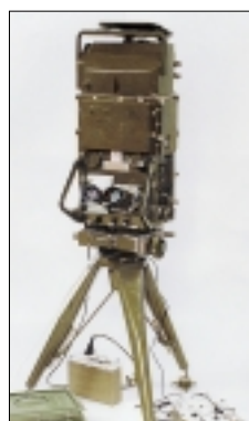
ЛЦД-1Д22 1D22 laser ranger designator
