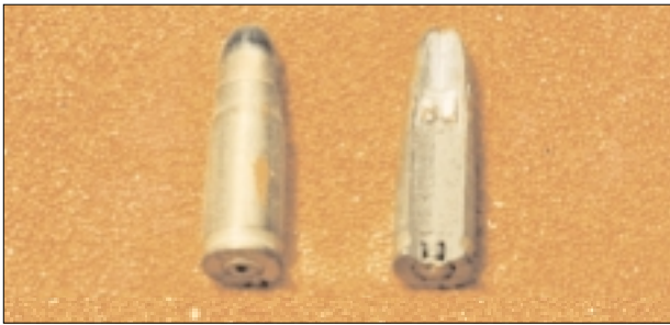
7.62mm PISTOL CARTRIDGE WITH TRACER BULLET (DESIGNATION 57-T-133 OR 57-T-132)
